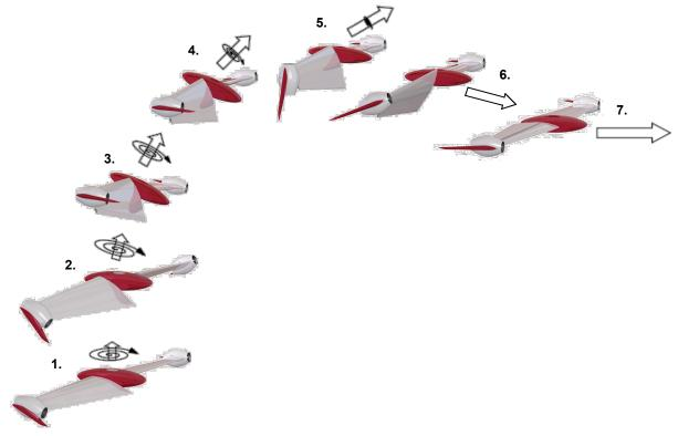
As its horizontal velocity decreases to a stall, the blades and engines orient down, and transition to vertical flight mode is initiated with a flap pulse that causes blade rotation, and stabilized with camber adjustments as the engines increase rotational velocity.
