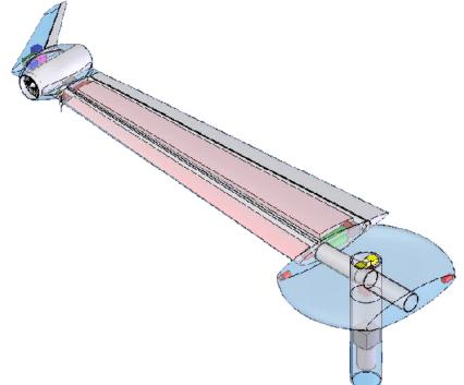
This eliminates the costly maintenance and failure associated with swash plates, shaft seals, and the counteraction of engine torque typical of Vertical Take-Off and Landing (VTOL) designs. Completely separating the transportation system from its payload makes the applicability of the Blade Flyer virtually unlimited. It is fully scalable from miniature Unmanned Air Vehicles (UAVs) to heavy left vehicles.
